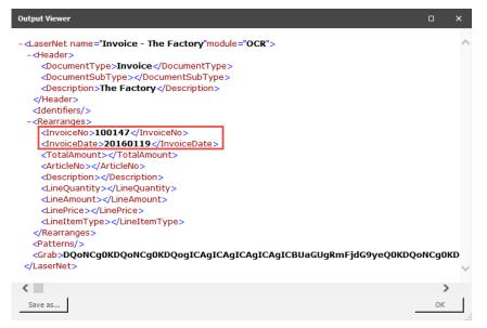
The date value is now added to the XML structure and converted to a standard format **yyyyMMdd** which is readable by most workflow systems.
